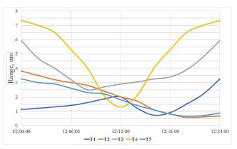
Fig. 10. Dynamic of changing range to five target ships throughout the experiment.
