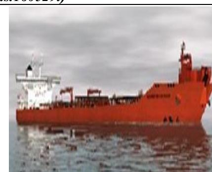
The vessel is equipped with one engine, Controlled Pitch Propeller (CPP), stern steering and bow thruster. CPP allows to change the screw force without changing the engine revolutions, but change of screw pitch and engine revolutions lead to a change in screw force and parameters of longitudinal movement and cannot be considered as two independent controls. In the
