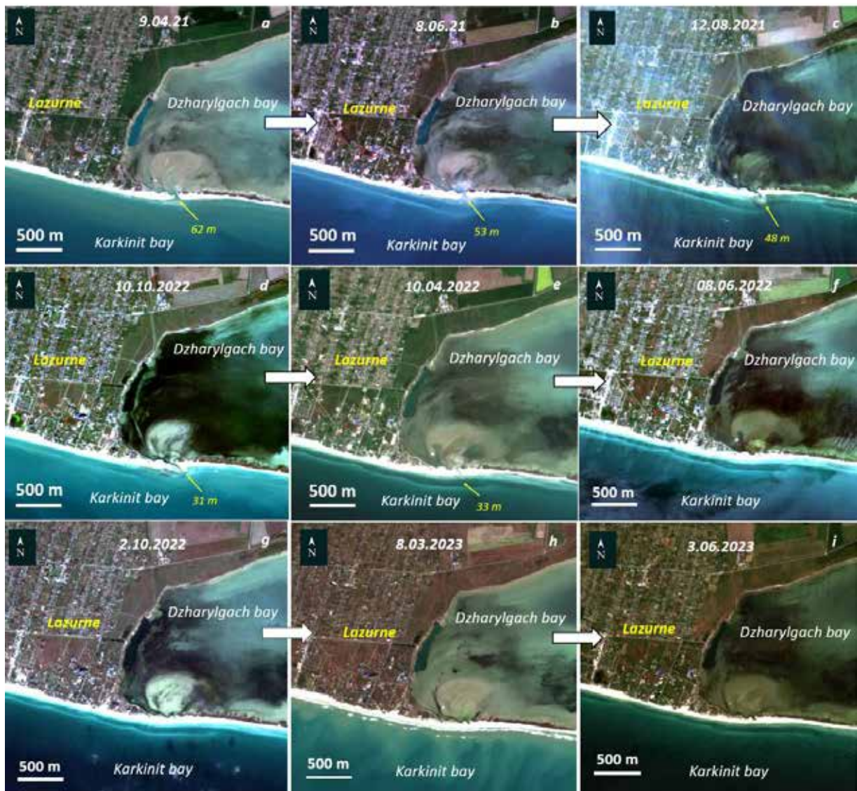
Fig. 3. Chronology of recent changes in the region of Lazurnenska Prorva: a – open (width: 62 m), April 2021; b – open (width: 53 m), June 2021; c – open (width: 48 m), August 2021; d – open (width: 31 m), October 2021; e – open (width: 33 m), April 2022; f – closed, June 2022; g – closed, October 2022; h – closed, March 2023; i – closed, June 2023 (yellow values refer to channel width; image source: Land Viewer)
