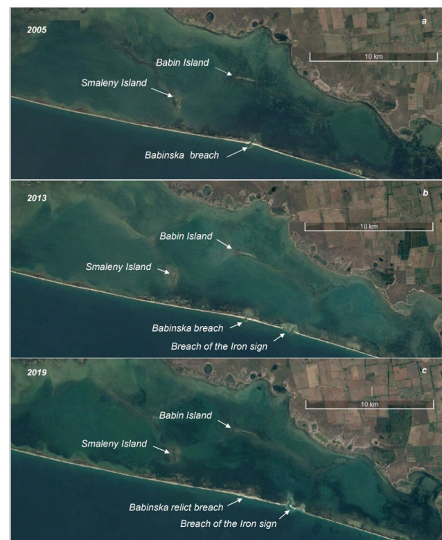
Fig. 8 Babinska breach and Iron Sign breaches during 2005–2019: a – stabilization of Babinska breach location; b – formation of a new breach in the vicinity of Iron Sign; c – closure of Babinska channel and an increase in complexity of the Iron Sign breach (based on Google Earth )
