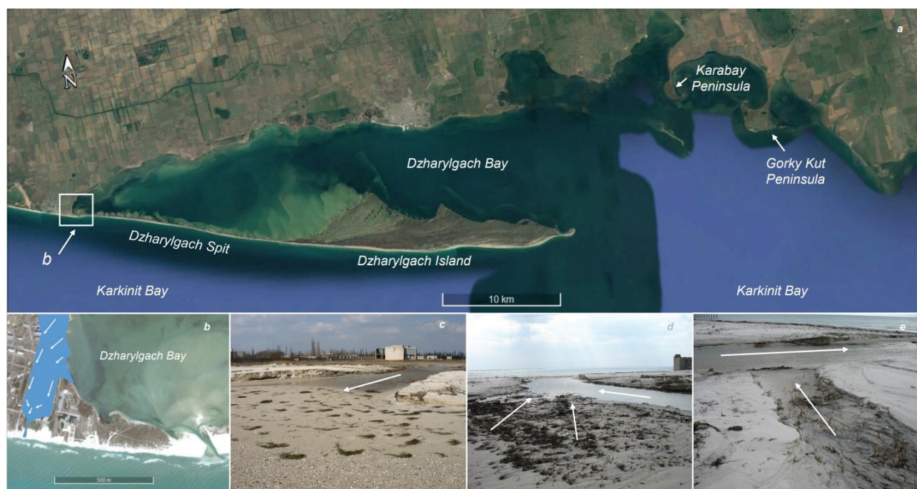
Fig. 10 Breach formation near the attachment (root) segment of Dzharylgach Spit complex: a – Lazurnenska prorva and washout into Karkinit Bay to the west; b – formation of the washout; c – view landward; d – view seaward; e – lateral spillover channel (arrows show principal water flow directions; satellite images: Google Earth; field photos by author: AD)
